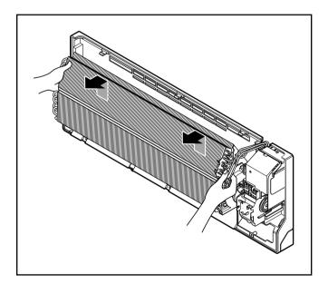
• Unhook the tab on the right inside of the chassis at the same time, slightly pull the evaporator toward you until the tab is clear of the slot.
